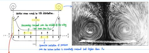
Hence, the surface pressure on the top surface of the delta wing is reduced near the leading edge
