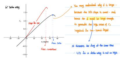
· Therefore, the aerodynamic effect of these vortices is not necessarily advantageous.
